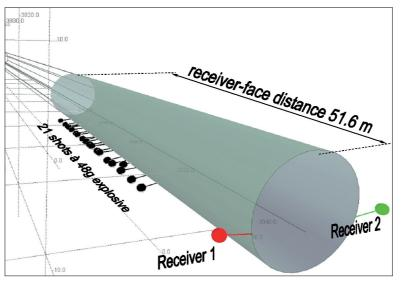
Receiver-shot layout of the TSP survey consisting of 21 shot holes each charged with 48g explosive along the left tunnel side wall.
