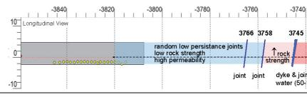
TSP result in longitudinal view (top) and observed geology after excavation of the predicted area.
