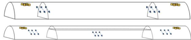
Figure 14 Installation of anemometers in Swiss road tunnels, with longitudinal ventilation (top) and smoke extraction (bottom)
