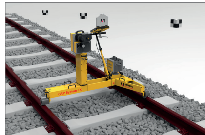
Absolute as-built track and infrastructure survey
