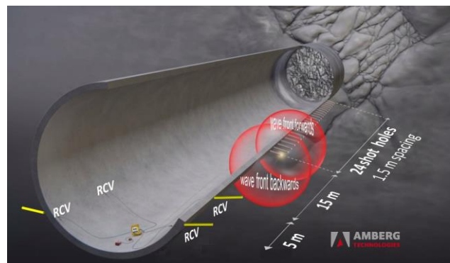
Figure 3. Measurement layout of the 3D Tunnel Seismic Prediction method consisting of usually 4 receivers (RCV) and 24 shot points.
