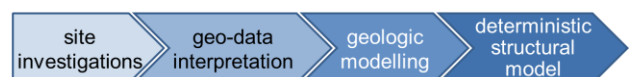
Figure 1. The conventional subsurface analysis workflow produces a single deterministic structural model of the ground.
