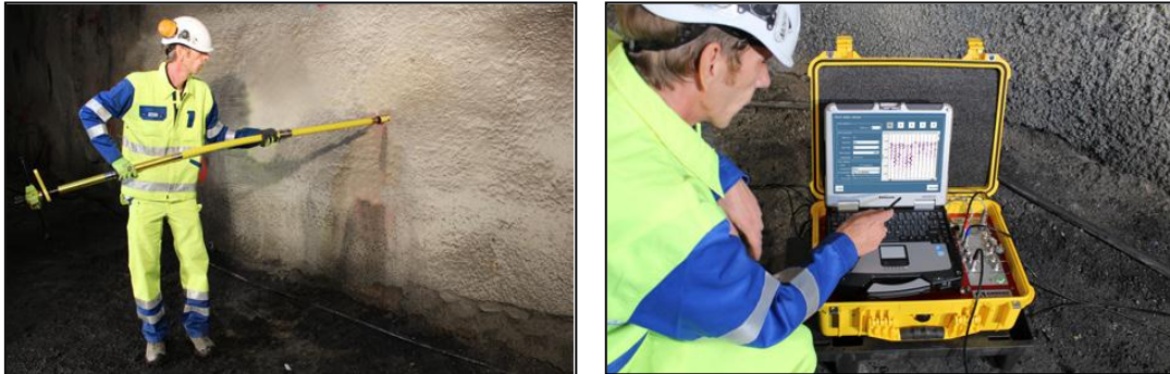
Figure 2. Simple installation of receiver and recording units of the TSP 303.
