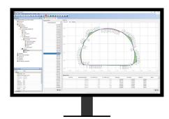
Amberg Profile enables you to quickly and efficiently analyze as-built tunnel profiles against the theoretical design. The module manages large quantities of profile data with ease, instantly converting measurements into comprehensive reports. Whether you're importing data from Amberg Navigator Tablet, Amberg Applications, or other sources, Amberg Profile simplifies the analysis process and ensures that your results are both accurate and easy to interpret.
