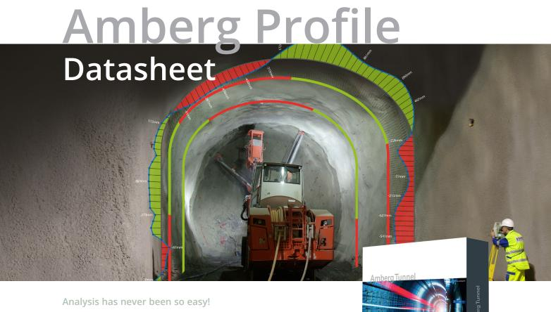
Amberg Tunnel's Profile Module instantly converts measurements into results. All reports are easy to understand and tailored to tunnelling needs. Using Amberg Navigator or Amberg Applications for measurements guarantees a seamless workflow. This ensures trouble-free data transfer of measurements from the tunnel into the office and vice versa (e.g. for layer thickness analysis).
