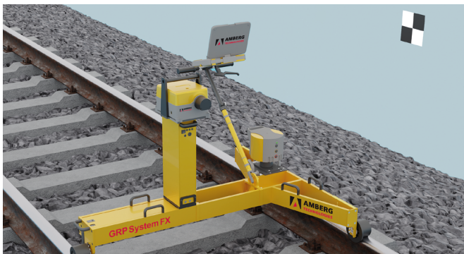
Absolute track geometry and infrastructure survey
