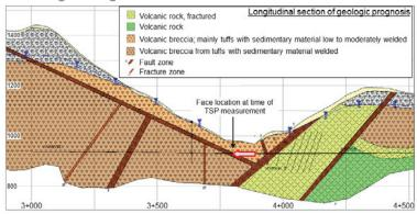
The extension involves excavating a tunnel parallel to the existing tunnel built in 1967. According to geological documentation of the prior tunnel, the overall quality of the massif could be seen as favourably though the excavated rock mass was composed of volcanic rocks with mainly weak characteristics revealing 15 fault zones. Temporary steel arches support of approximate 30% of tunnel length was being supposed.
