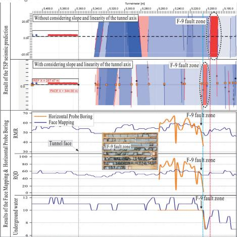
On the other hand, the horizontal probe drilling and surface observation during the tunnel excavation showed that the F9 fault zone already started from STA. 5+207.0, which differs by about 10 m from the TSP results. The main cause of the location error was judged due to the downward excavation, with the slope gradient of 4.95 %.
