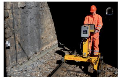
Laser scanner set up on trolley with fixed point for measuring on the tunnel wall.
